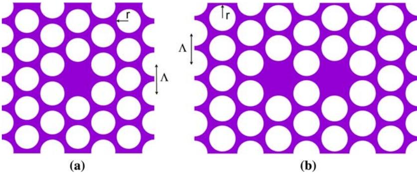
**Fig. 2** Sketch of a photonic crystal fiber (PCF) structure (transverse plane) with a triangular lattice geometry. (a) Single-core PCF; (b) dual-core PCF coupler.  $\Delta$  and  $r$  are respectively the pitch (distance between holes) and hole radius, which characterize the structure
