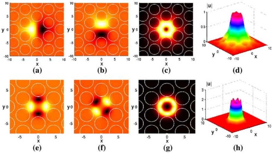
**Fig. 5** Vortex states in a photonic crystal fiber. Top row: linear vortex for  $\ell = 1$ , (a–b) dipole field, (c–d) vortex field. The calculated propagation constant is  $\beta = 1.18$ . Bottom row: nonlinear vortex for  $\ell = 2$  and  $\beta = 3$ , (e–f) quadrupole fields, (g–h) vortex field
