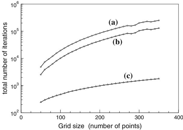
**Fig. 8** Performance comparison between the modern solver (SYMMLQ) and two of the classical solvers (Jacobi and Gauss-Seidel) for the calculation of the lowest state of the linear dual-core PCF coupler, using the inverse iteration method: (a) Jacobi, (b) Gauss-Seidel, (c) SYMMLQ
