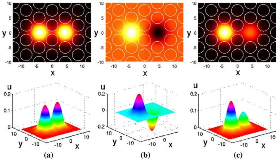
**Fig. 3** Two dimensional (top row) and three-dimensional (bottom) plots of different stationary states of a nonlinear dual-core photonic crystal fiber coupler. (a) Symmetric, (b) antisymmetric, (c) asymmetric. Parameters were chosen as  $\Lambda = 5$  (pitch),  $r = 2$  (hole radius),  $n_s = 1$ ,  $n_a = 0$  and  $\beta = 0.74$
