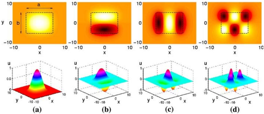
**Fig. 1** Some of the different stationary states (modes) of a linear rectangular waveguide with a core of refractive index  $n = 3$  in a substrate of  $n_s = 1$ . Core dimensions are  $a = 8, b = 6$ . Propagation constants for the states  $\beta_{\nu\mu}$ , where  $\mu$  and  $\nu$  indicate the number of nodes in each direction, are (a)  $\beta_{00} = 2.7126$  (fundamental mode), (b)  $\beta_{01} = 2.1961$ , (c)  $\beta_{20} = 1.8623$  and (d)  $\beta_{21} = 1.3702$
