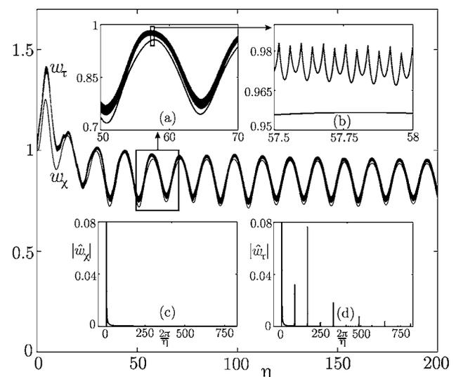
Fig. 2. Oscillations of the spatial (lower) and temporal (upper) widths of the stabilized soliton with  $g=1.074g_c$  from Fig. 1. (a) and (b) Insets display details of the curves. (c) and (d) Insets show the frequency spectra of the spatial and temporal width oscillations, respectively.
