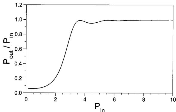
Fig. 4. Switching curve calculated for the PCF nonlinear coupler of Fig. 1(b). Due to the stability of the asymmetric mode and the instability of the symmetric one, the light launched into one core only does not switch to the second core but remains in the same core.
