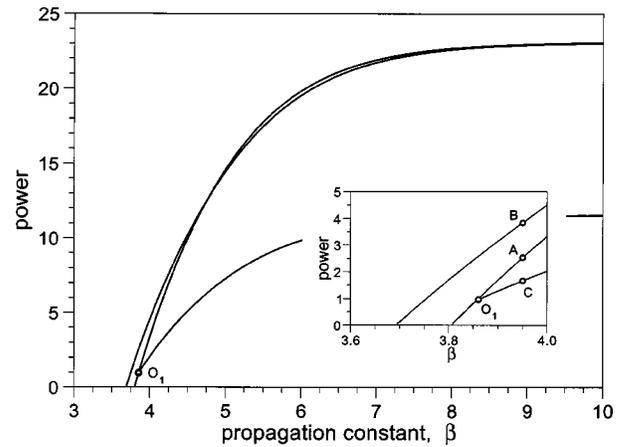
Fig. 3. Bifurcation diagram of the coupler modes. Inset, enlarged part near the bifurcation point. Asymmetric mode C bifurcates from symmetric mode A at point  $O_1$  above a certain threshold in the mode power.
