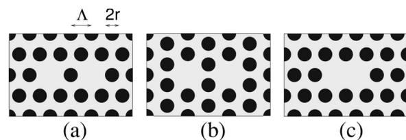
Fig. 1. Schematic of three studied designs of a nonlinear dual-core PCF. The coupler is created by two missing neighboring holes in a nonlinear material.
