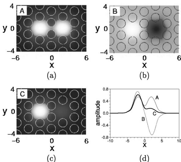
Fig. 2. (a)–(c) Light distribution between the two PCF cores in Fig. 1(b) for three distinct nonlinear modes: A, symmetric; B, antisymmetric; and C, asymmetric. (d) Transverse profiles of the nonlinear modes ( $\beta=3.95$ ).
